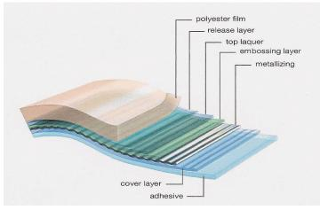
Figure 1 b; a cut away view of an OVD foil
